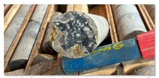
Figure 1: Drill core from resource diamond drill hole ST23-02 showing chalcocite (dark grey) copper sulfide breccia at approximately 354.7m downhole.
