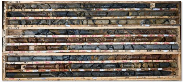
TAT23-002 drill core from the mineralized section (147.1 to 161.0 m). Scintillometer readings are written on the core boxes in counts per second and were measured using a digital, hand-held CT-007M scintillometer by Environmental Instruments Canada
